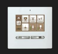
THE HIP-100 (above) user interface by Lagotek installs directly in the wall in lieu of a 2-gang light switch. The touch panel controls most elements in a total home system. "Modes" can be set for each user or for times night or vacation.
